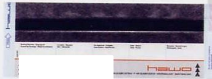
1. Intact seal for a specified seal width in accordance with EN ISO 11607, Part 2
